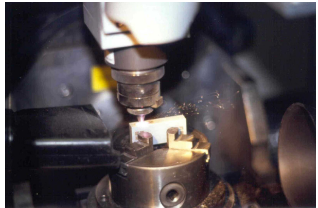
Development of smoke during laser-beam machining
